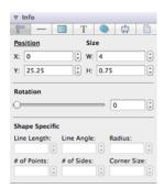
If you look closely, you'll notice that the stairs overlap the exterior walls slightly. Use the Fill Tab in the Info Panel of the sidebar to turn off the fill visibility for this shape and make it visually cleaner. Click on the Fill Visibility toggle to disable (uncheck) this option.
